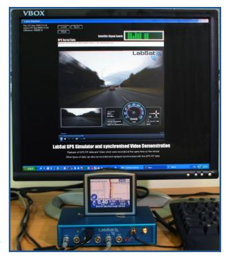
LabSat replays a test drive through a SatNav alongside synchronised Video VBOX video, providing developers with information about real world conditions encountered during recording.
